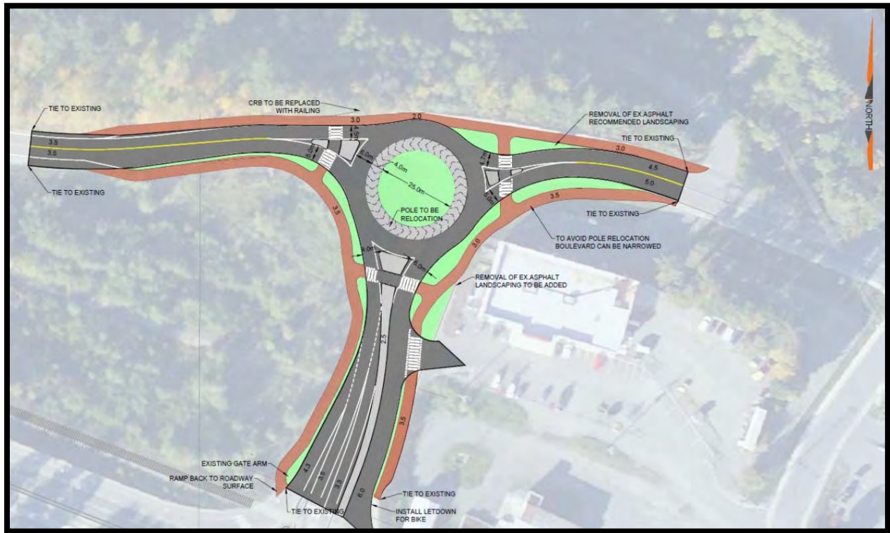
Figure 4: Ludlow/Rocky Creek Road Roundabout Design
