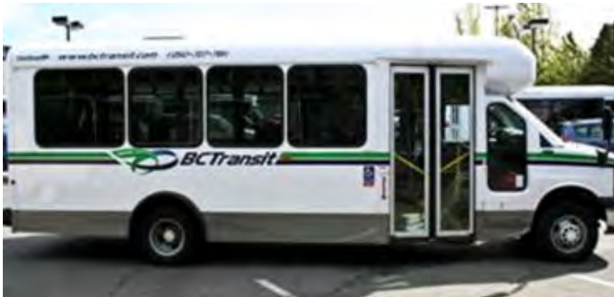
Arboc Length: 8.05m Width: 2.41m Height: 3.02m Side door ramp deployment dimensions??
