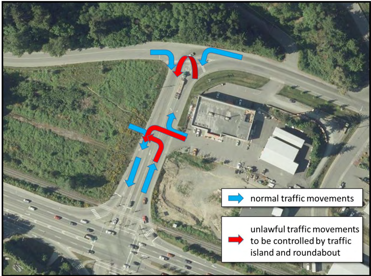
Figure 3: Existing Traffic Movements at Ludlow/Rocky Creek often require U-turns or unlawful left turns onto Ludlow
