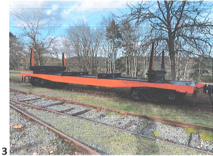
1, 2: Rustproofing lower works after rust descaling. 3: Log car with painted upper and lower works.
