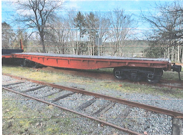
Bull car showing decaled, rust proofed and newly painted upper and lower works and new wooden deck.
