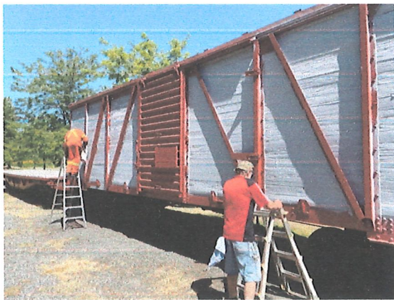
1: Applying undercoat to caulked exterior boards 2: Box car red final coat applied. Awaiting decals.
